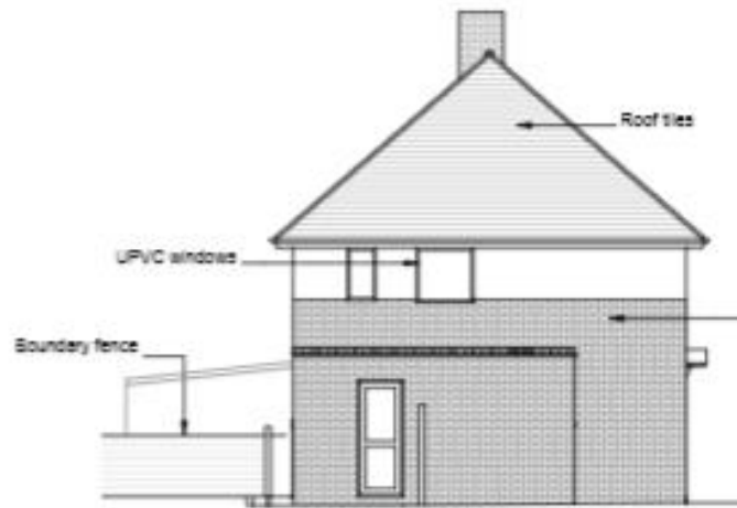
Existing Side Elevation 1:100
